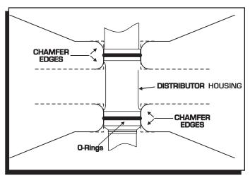
Figure 9 Modified Block for use with 0-Rings.
