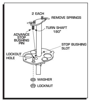
Figure 7 Locking Out the Advance.
