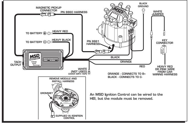
Figure 11 Wiring to an MSD Ignition Control.
