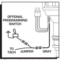
Figure 14 Setting the Rev Limiter.
