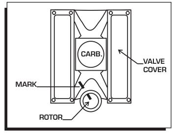
Figure 8 Marking the Rotor Location.
