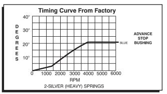
Figure 2 The Factory Equipped Curve.
