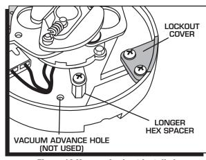
Figure 13 Vacuum Lockout Installed.
