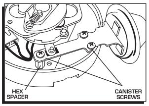
Figure 12 Removing the Vacuum Canister.
