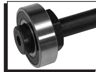
Figure 8 Installing the New Bearing.
