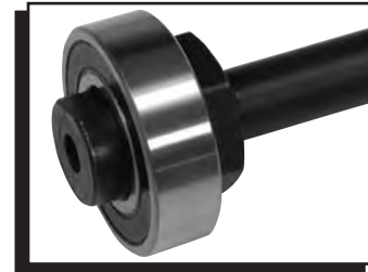
Figure 8 Installing the New Bearing.
