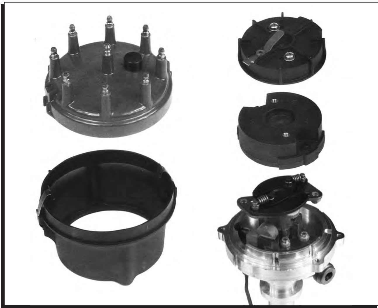
Figure 3 Installing the Cap-A-Dapt.
