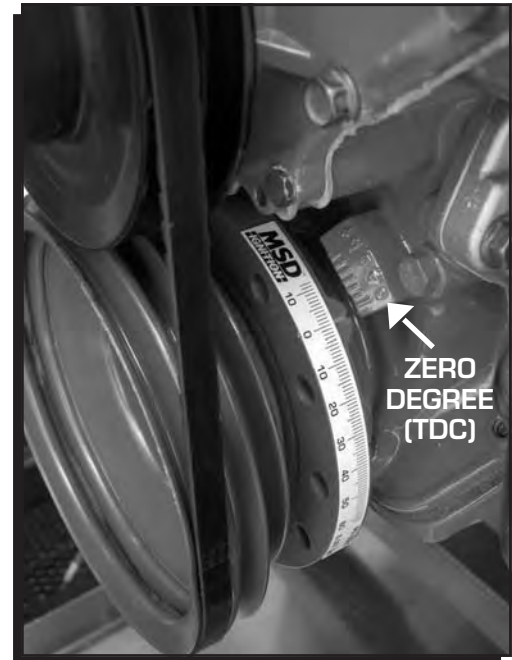
Figure 8 The Timing Tape Installed.
