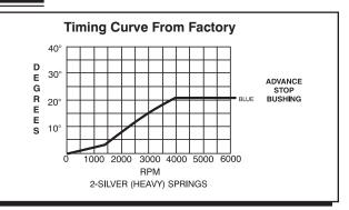
Figure 2 The Factory Equipped Curve.
