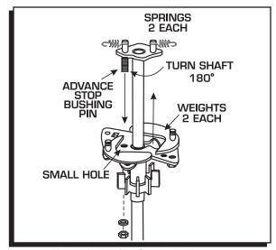
Figure 8 Locking Out the Advance.
