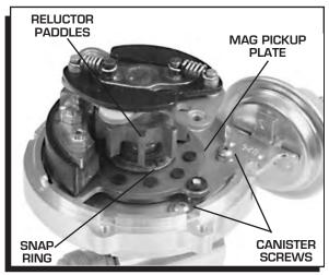
Figure 10 Removing the Vacuum Canister.
