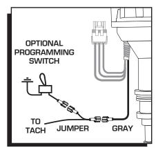
Figure 14 Setting the Rev Limiter.
