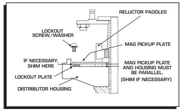
Figure 11 Checking Installation of the Lockout Plate.
