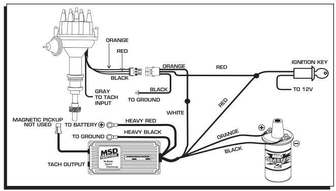
Figure 13 Wiring to an MSD Ignition Control.
