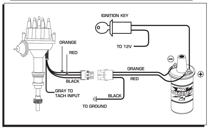
Figure 12 Wiring the Ready-to-Run Distributor.
