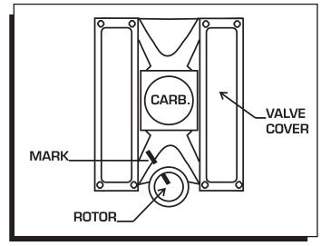
Figure 9 Marking the Rotor Location.
