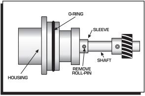
Figure 7 Removing the Retaining Sleeve.
