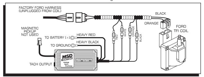
Figure 2 Installation with an MSD 6 or 7 Series Ignition Control.
