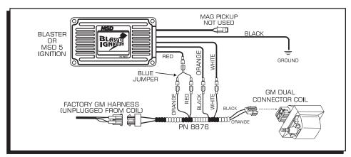
Figure 4 Installation with an MSD 5 or Blaster Ignition.
