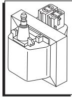
Figure 1 GM Dual Connector Coil.
