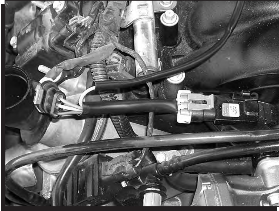
Figure 2 Map Sensor Connection.
