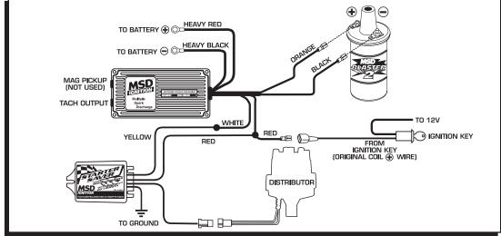
Figure 1 Wiring the Control with an MSD 6 Series Ignition Control.
