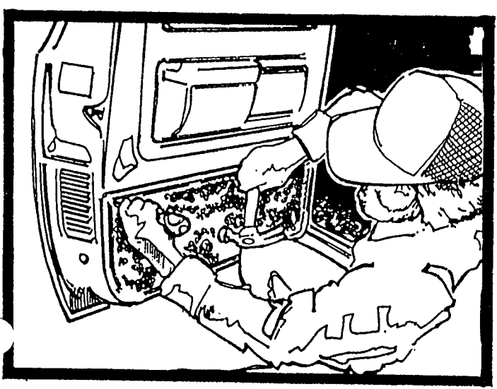
STEP 2 USE PRE-MADE HOLES AS GUIDE, WITH AWL MAKE HOLES FOR SCREWS
