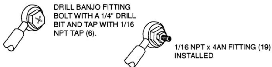
Figure 13 Schematic of “Drilled Out” Banjo Fitting
