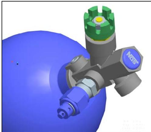
5. Carefully use a straight blade screw driver to quickly crack the valve open and closed. Be very careful not to expose skin or eyes to nitrous spurt if there are no attachments on the bottle opening. This step is to ensure that the bottle valve was not over torqued and too tight for the motor to open.
