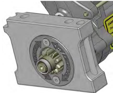
**Using Blue Loctite® or equivalent thread lock on the two ring bolts is REQUIRED!**
