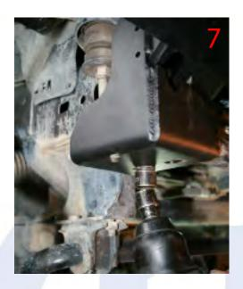
• Install the winch to the bumper using the supplied Allen Bolts and Washers.
