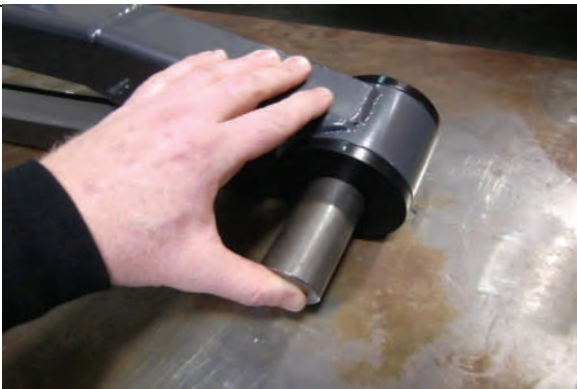
Stage 2 Lube pivot pin and install into bushings
