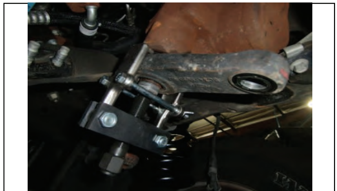
Use proper pitman arm puller to remove from steering box
