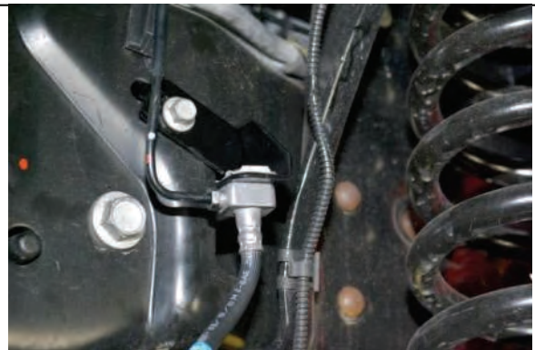
Reinstall block into bracket with retaining clip.
