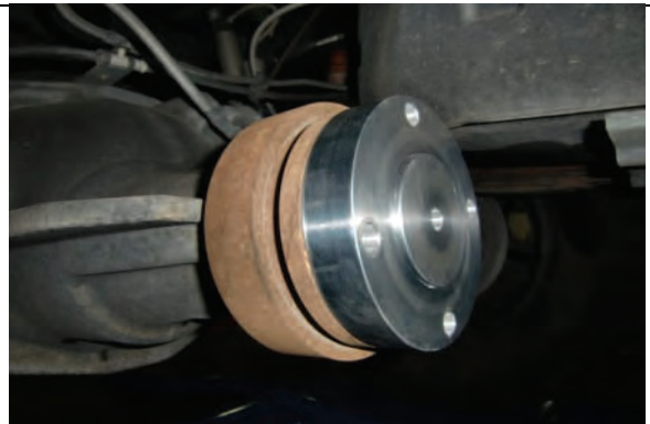
Clean off mount and ensure spacer fits flush
