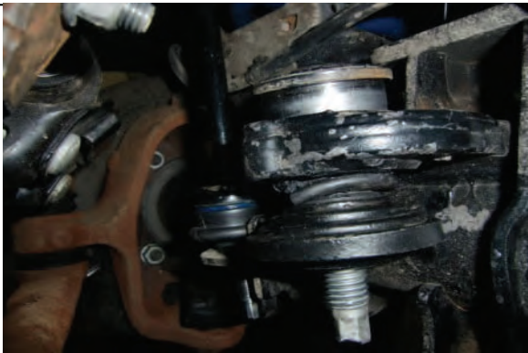
Remove ball joint from axle
