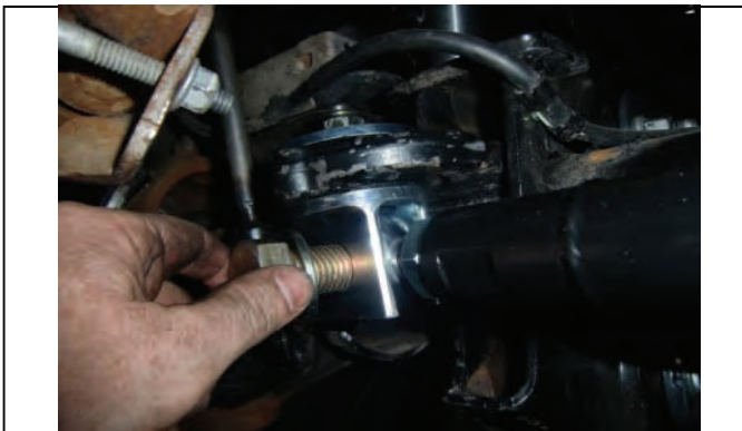
Attach with provided hardware, do not tighten until adjusted
