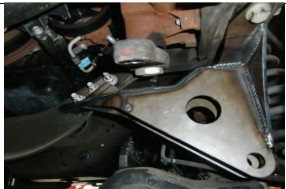
Install new track bar drop bracket w/ OE fasteners, torque
