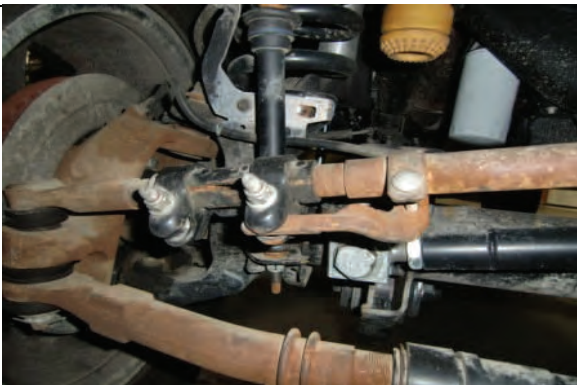
Tighten up hardware and replace keeper bolt
