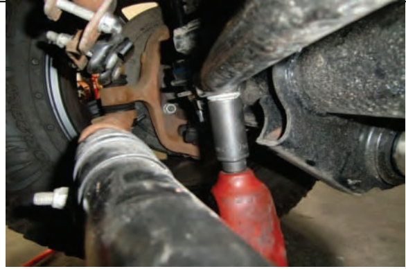
Loosen ball joint nut and leave attached
