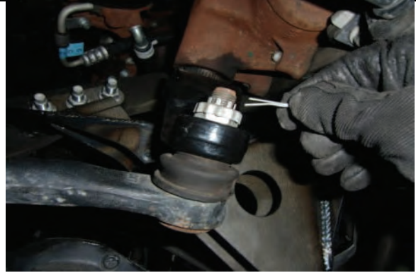
Replace keeper cap and cotter pin.
