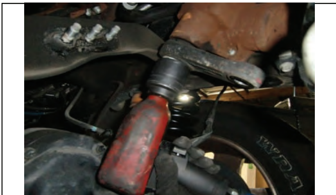
Remove pitman arm nut
