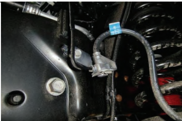
(11-up) models replace OE bracket with new drop bracket.
