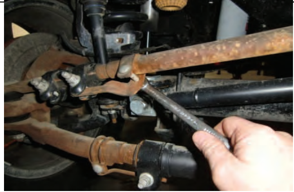
Remove safety keeper bolt and slide bracket out of collar
