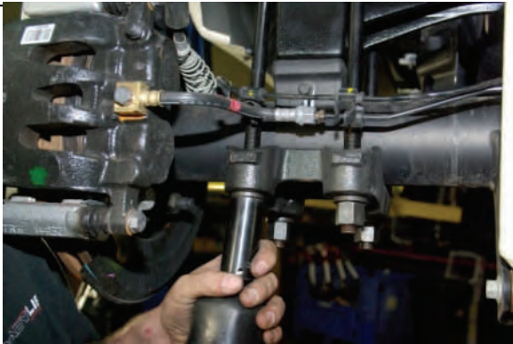
Loosen and remove OE u-bolts and nuts from leaf pack
