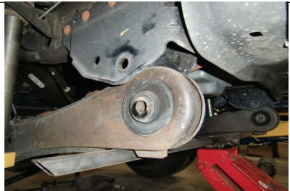
Carefully lower radius arms enough to install drop brackets
