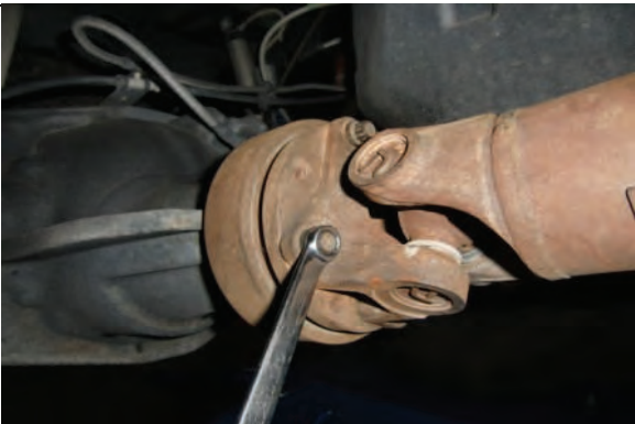
Vehicles w/1pc drive shaft, remove (4) bolts at differential
