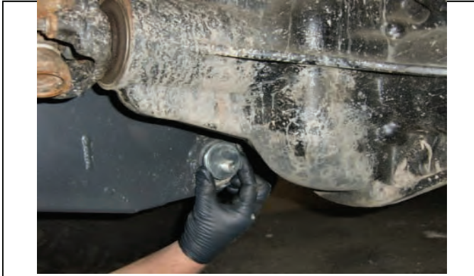
Stage 2 Install new offset cams/bolts/nuts in lower mount
