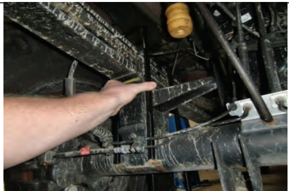
Install new u-bolts and hardware around axle and secure
