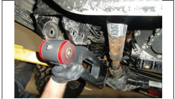
Stage 2 Raise radius arm into frame, attach w/ OE hardware
