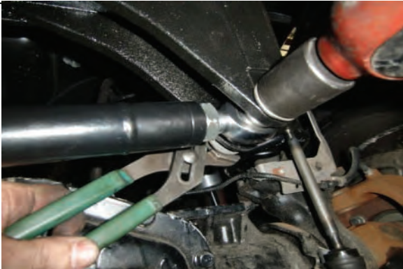
Tighten other end at frame mount to OE spec
