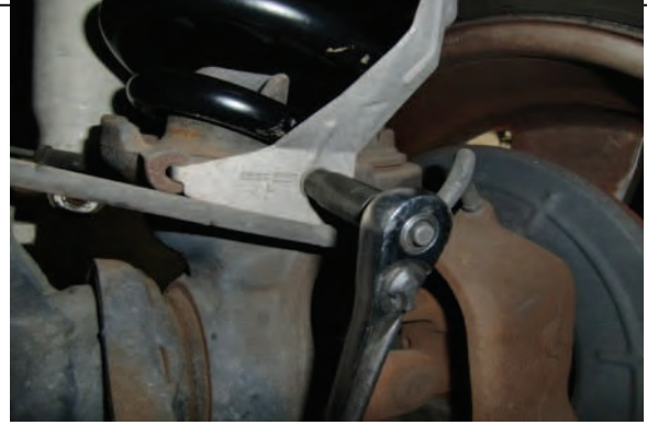
Disconnect brake line bracket from lower spring perch
