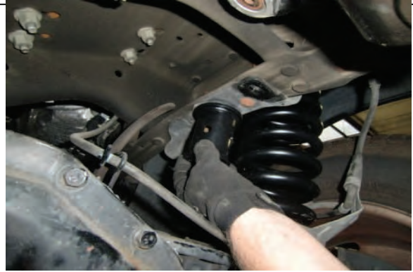
Screw bump stop drop bracket into OE frame location
