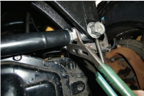
Tighten jam nut at frame mount
