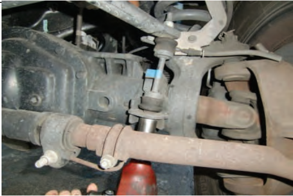
Disconnect and remove factory sway bar end links
