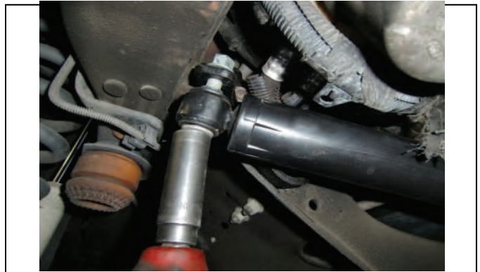
Disconnect steering stabilizer at the frame
