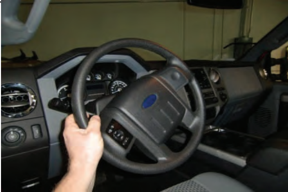
Straighten steering wheel steps, Unlock steering wheel
