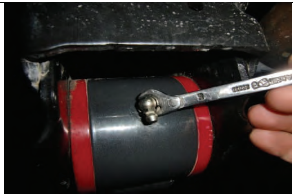
Stage 2 Install provided zerk fitting
