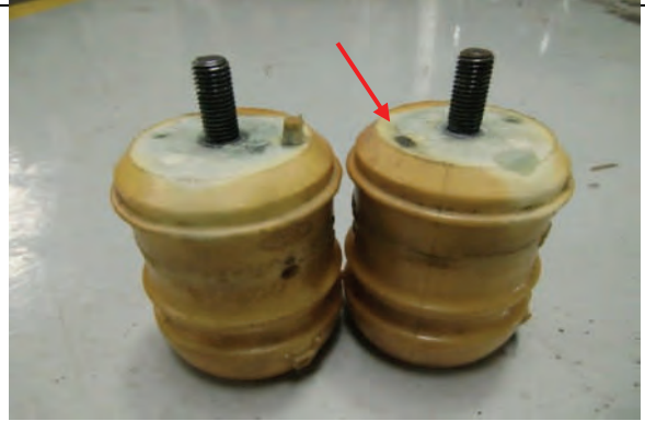
Note: Locating tab must be trimmed from bump stop
