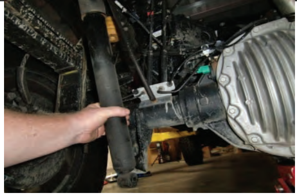
Remove rear shocks. Note: Longer shocks required
