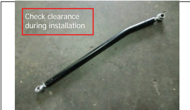
Use assembled track bar as a guide to ensure proper position
