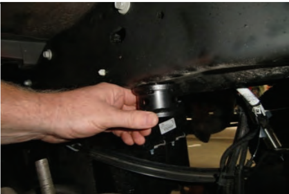
Install rear bump stop extension in OE location
