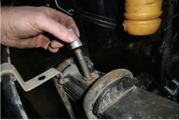
Install spacer tube and OE bracket over dr side centering pin
