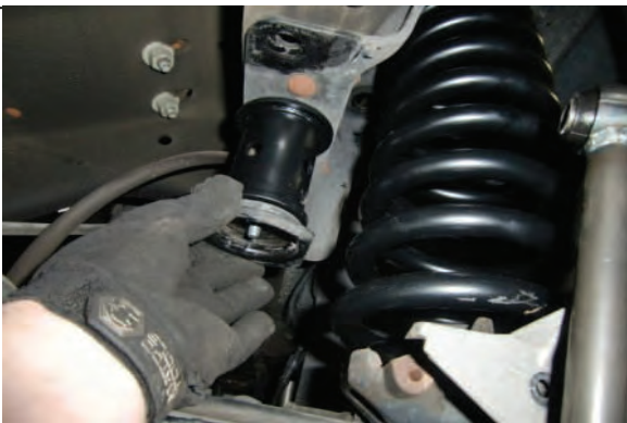
Reinstall/align OE bump stop cups onto drop bracket
