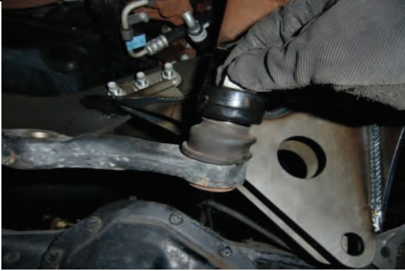
Reattach drag link to new drop pitman arm and torque
