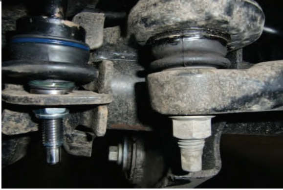
Stage 3 (Next 3 pgs.) Track bar ball joint at axle mount
