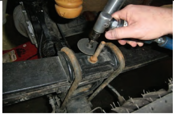
Cut off excess centering pin threads on pass side leaf pack
