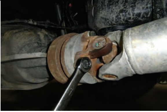
Install driveshaft spacer with new provided hardware, torque
