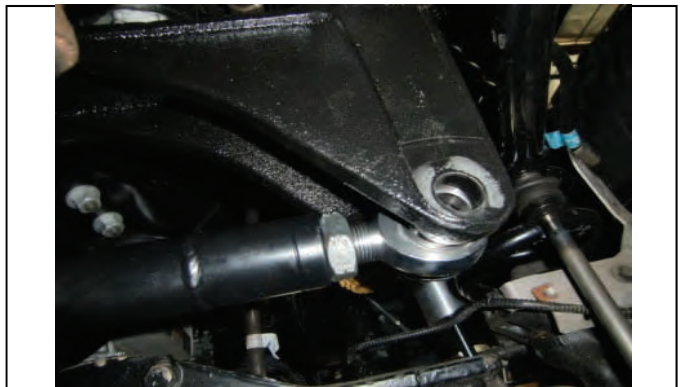
Position other end at frame w/ provided misalign spacers
