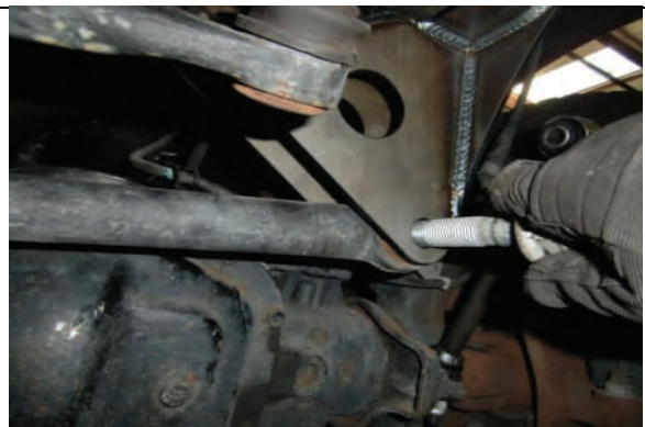
Reconnect track bar to drop bracket with OE hardware,
