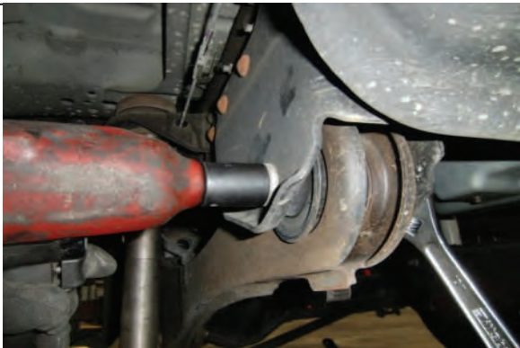
Loosen and remove bolts at rear of dr./pass. radius arms
