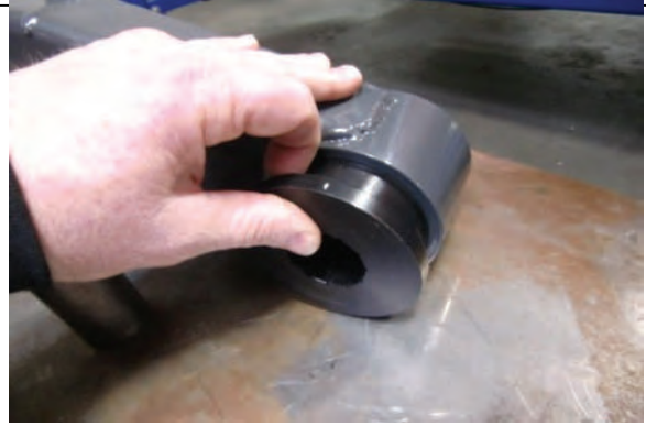
Stage 2 Use assembly lube to install urethane bushings
