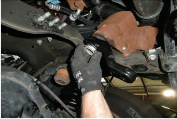
Install new drop pitman arm w/OE nut and torque to spec.
