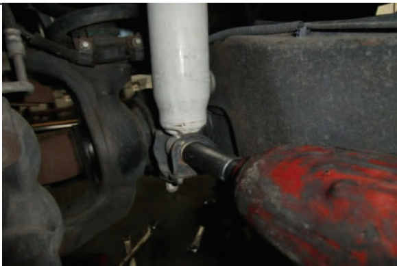
Remove front factory shocks, Note: longer shocks req'd
