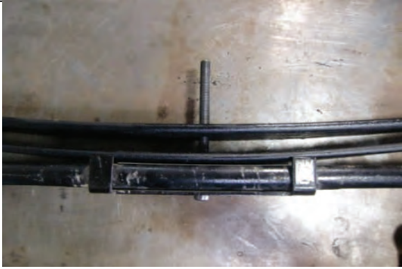
Place overload spring below add-a-leaves w/ new centering pin
