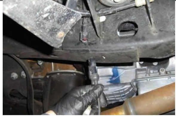
Disconnect ABS line at plug above radius arms
