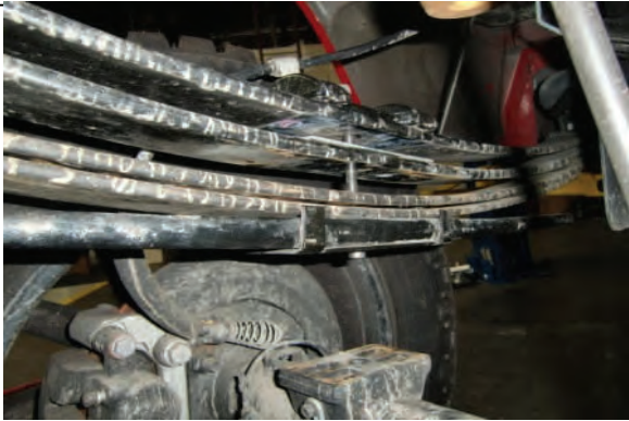
Clamp leaves together and torque new centering pin to spec
