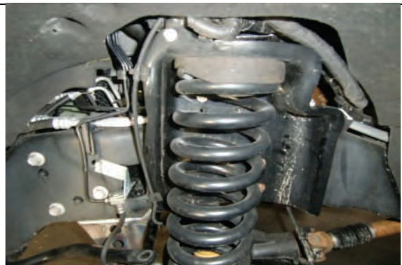
Lower vehicle down onto new springs and allow to settle
