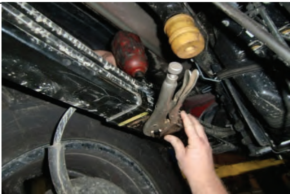
Clamp centering pin bolt, loosen bolt and support lower leaf
