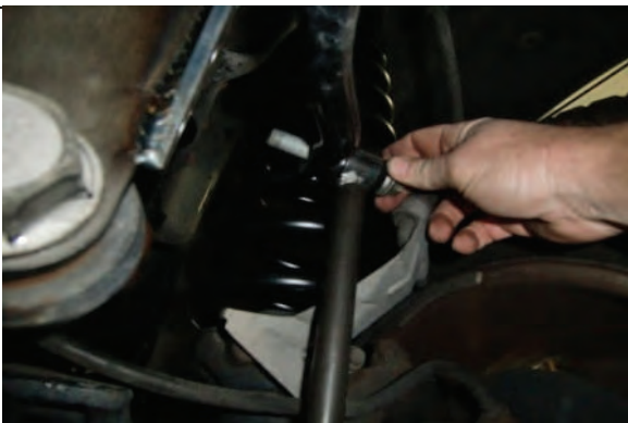
Attach top sway bar end link to sway bar
