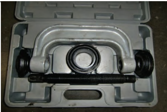
Use proper heavy duty ball joint removal tool set
