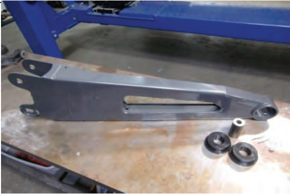
Stage 2 Gather radius arms and bushing kit for assembly
