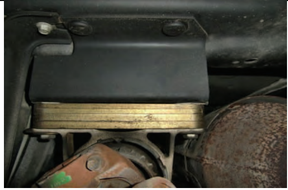
Vehicles w/2pc drive shafts may require drop carrier shims
