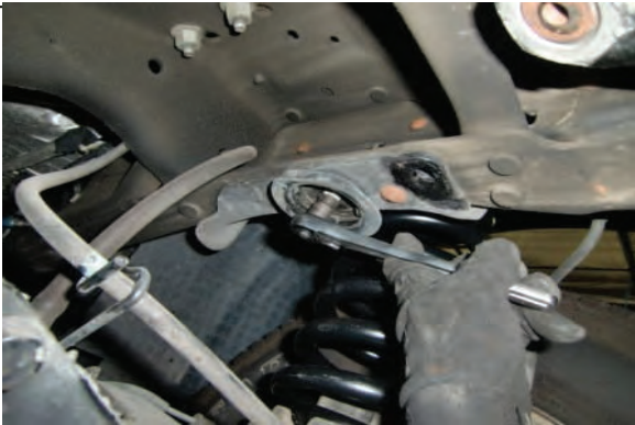
Remove bump stop cup mount from frame
