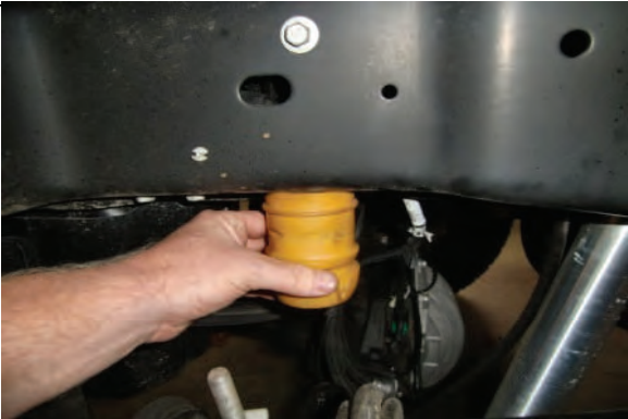
Remove rear bump stops from frame, nut inside frame
