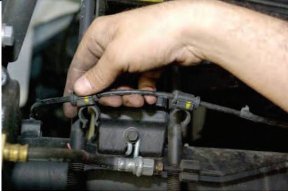
Disconnect ABS line clips from dr/pass side u-bolts
