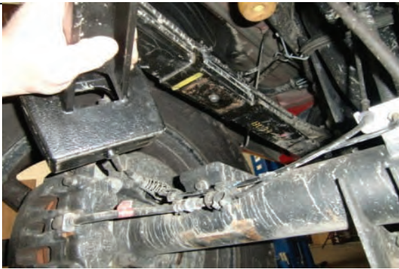
Lower axle and remove factory lift block
