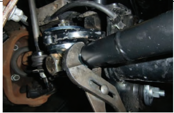
Tighten jam nut at axle mount
