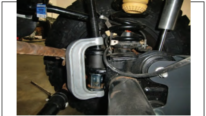
Use press tool to draw clevis into position
