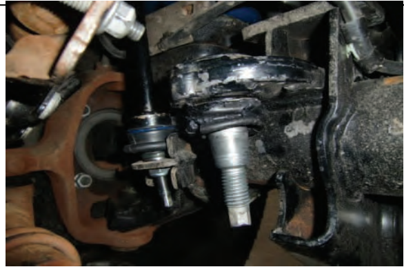
Shown, ball joint to be removed
