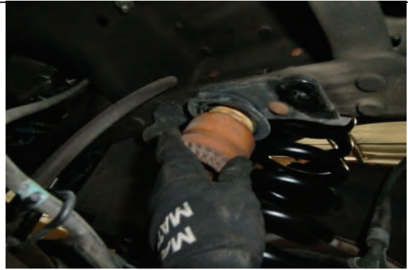
Remove front foam bump stops from frame
