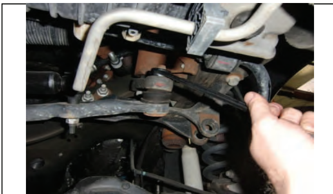
Remove cotter pin and disconnect drag link from pitman arm
