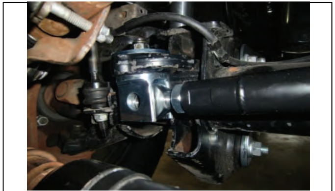
Insert track bar into clevis, check clearance
