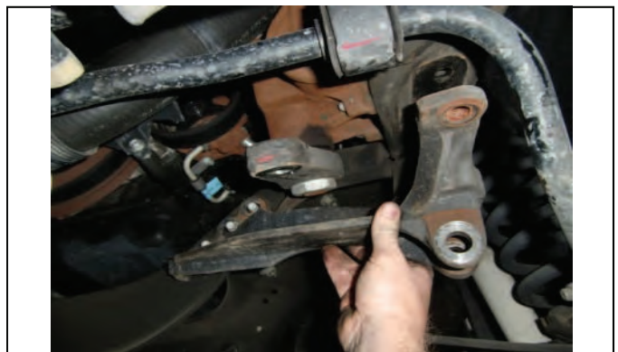
Remove factory track bar bracket from cross member/frame
