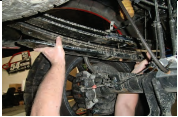
Install assembled leaves below main leaf pack
