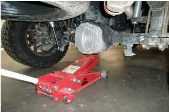
Rear Install: Lift rear of vehicle by frame and support axle
