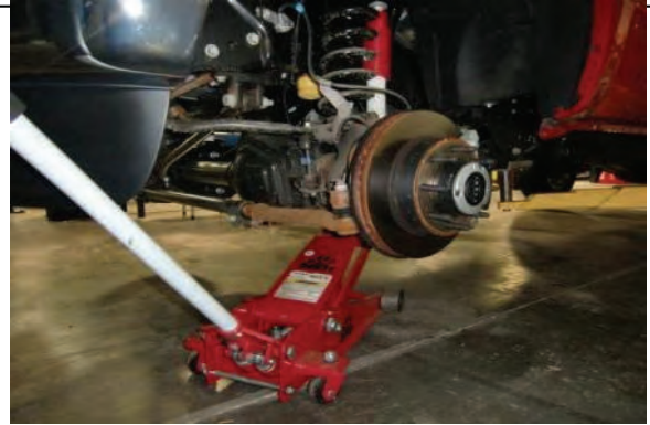
Remove front wheels and tires, support axle with jack stands
