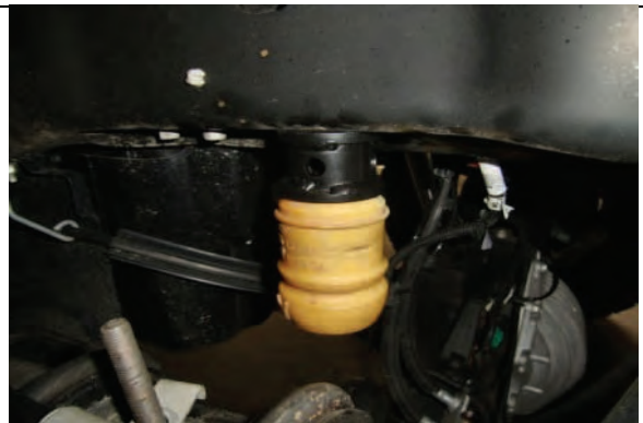
Reinstall OE bump stop on drop bracket
