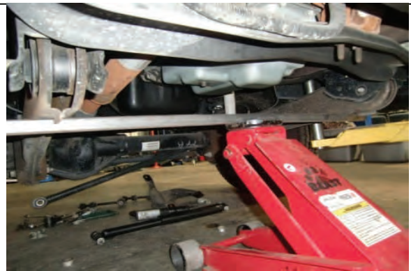
Use a floor jack and crossbar to support both radius arms
