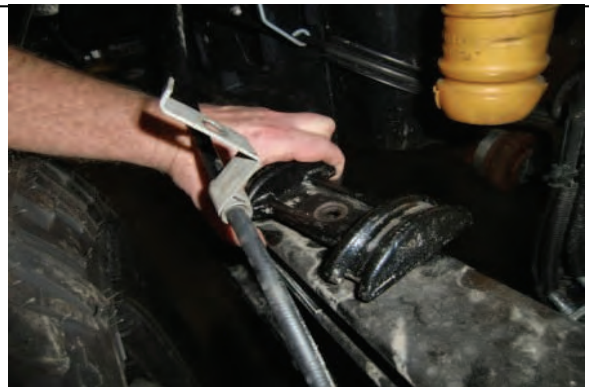
Remove upper u-bolt mounting plate
