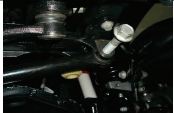
Remove upper track bar hardware and disconnect at frame.
