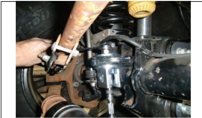
Tighten hardware to spec once clevis is properly seated
