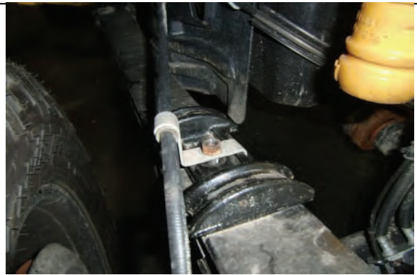
Dr side, remove e-brake bracket from upper u-bolt plate
