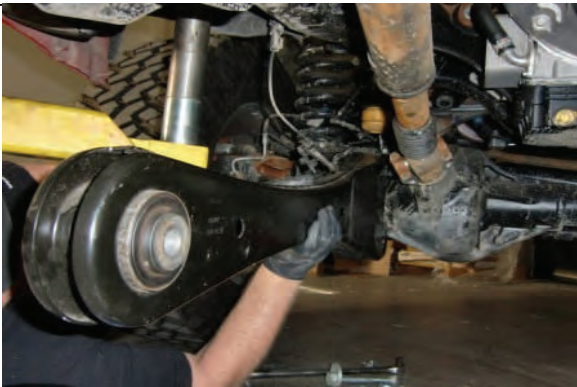
Stage 2 Remove front radius arm hardware and arm
