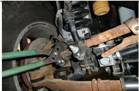
Adjust collar to straighten steering wheel
