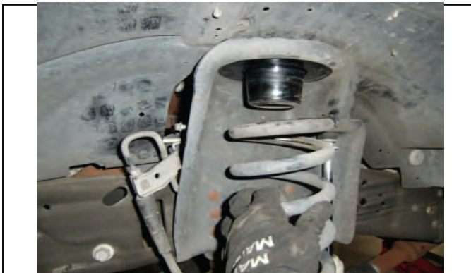
Slowly raise vehicle enough to remove factory springs
