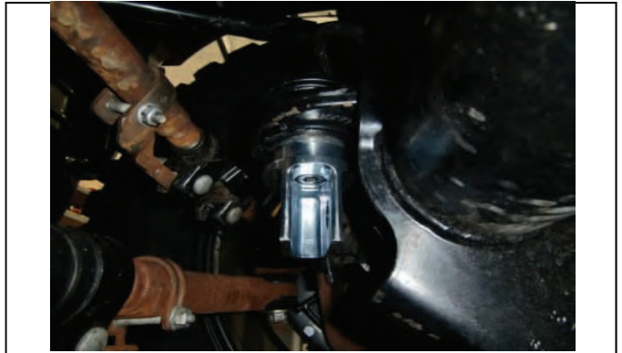
Align clevis so it lines up with track bar frame mount bracket
