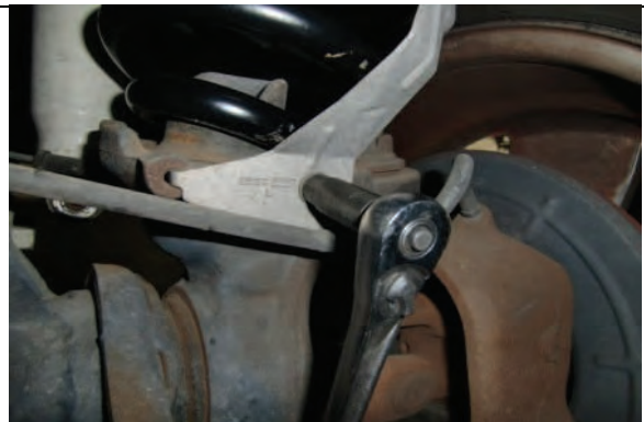
Reattach brake line hose/bracket to lower spring perch
