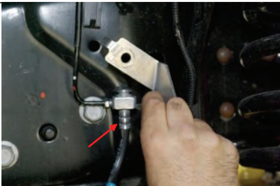
Note line direction, replace OE bracket with new drop bracket
