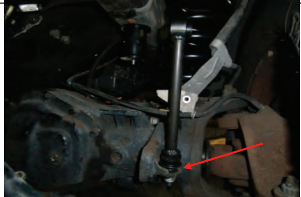
Install new end link into lower axle tab with new hardware
