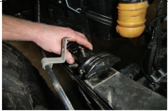
Place upper u-bolt mounting plate on top of centering pin
