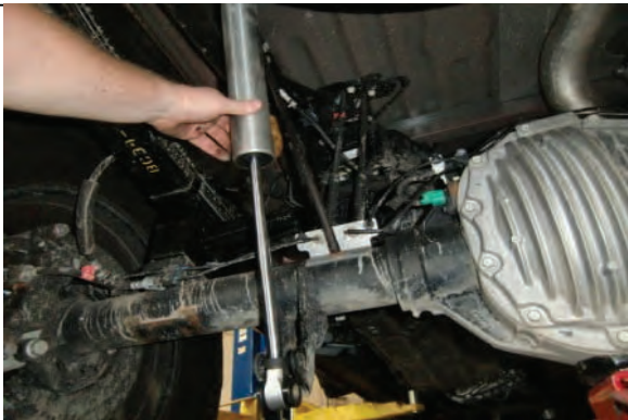
Install longer shocks and tighten to spec
