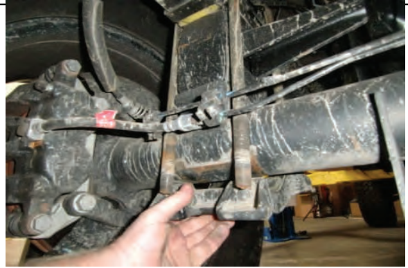
Remove u-bolts and lower axle plate
