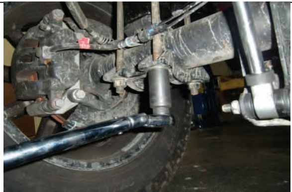
Lower vehicle to ground and torque u-bolts to spec
