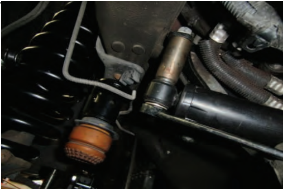
Install steering stabilizer drop boss and mounting hardware
