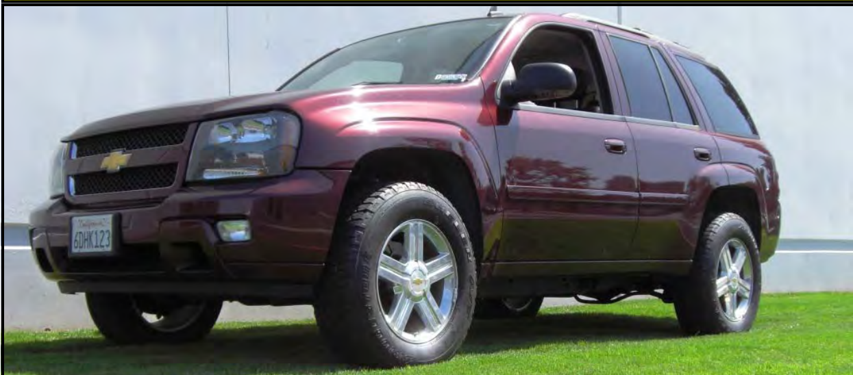
After ReadyLift SST Lift Kit 69-3065. 255/70R18 Bridgestone Dueler on 18x8 +50 offset OE wheel w/1.5" wheel spacers.
