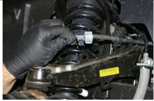
Unclip brake lines from upper control arms
