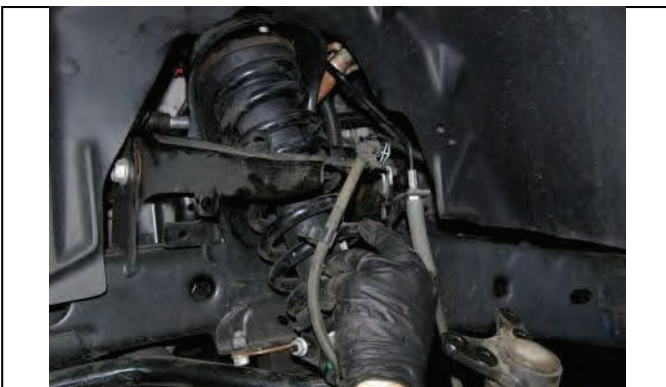
Remove upper strut mounting hardware. Remove strut
