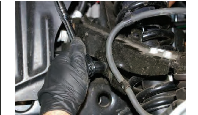
Disconnect brake line bracket from upper control arm
