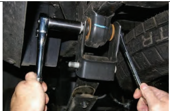
Disconnect and remove shackles
