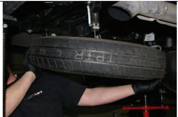
Remove spare tire to allow shackle bolt removal
