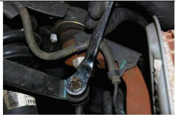
Disconnect and remove sway bar end links
