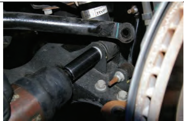
Remove lower strut mounting hardware
