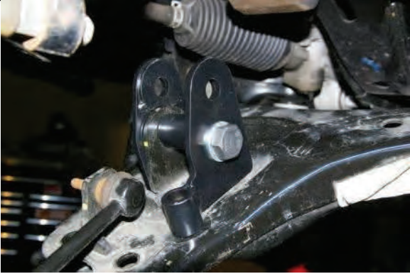
Assemble lower strut extension brackets as shown
