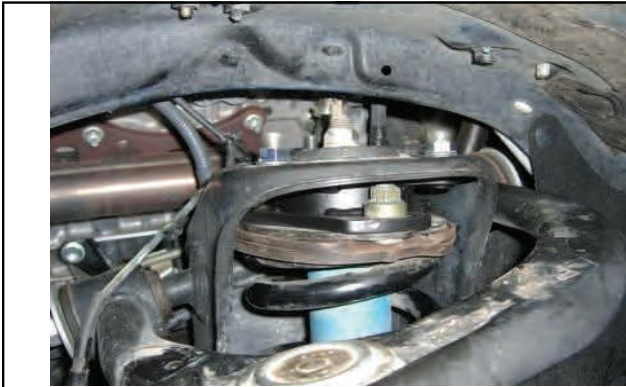
Rotate 180 deg., reattach upper strut with provided hardware
