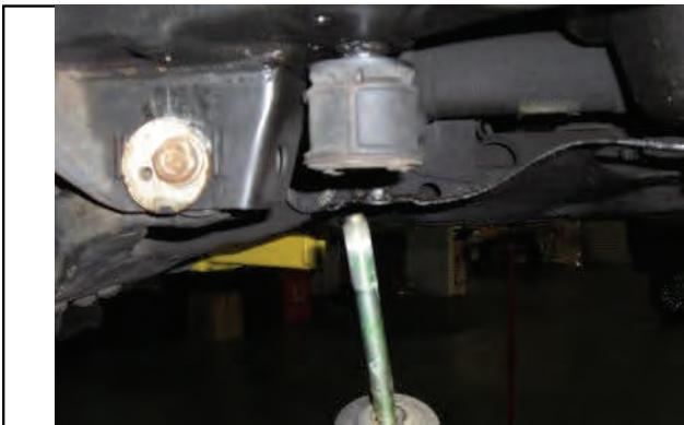
4WD Support differential and remove (2) front mounting bolts
