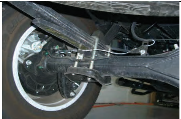
Work on one side at a time to prevent driveline damage.
