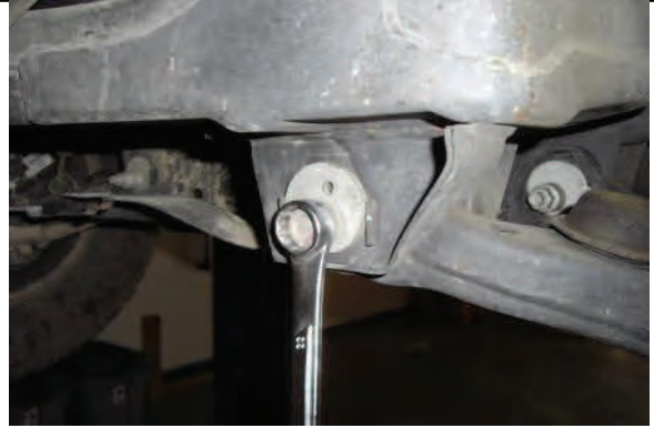
Reset and tighten lower control arm bolts
