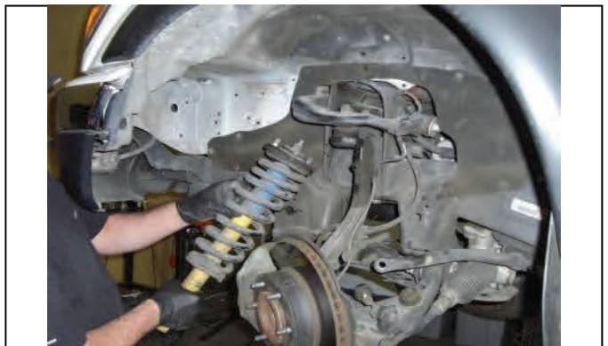
Remove strut from vehicle
