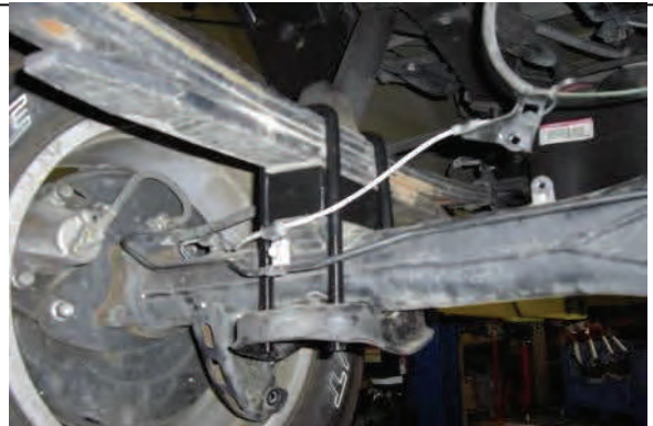
Attach lower mounting plate with provided hardware.
