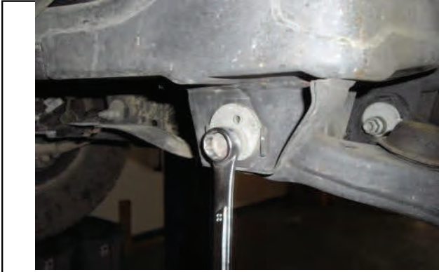
Mark and loosen lower control arm bolts, do not remove
