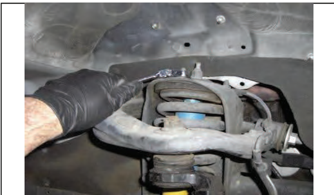
Disconnect upper strut mounting hardware
