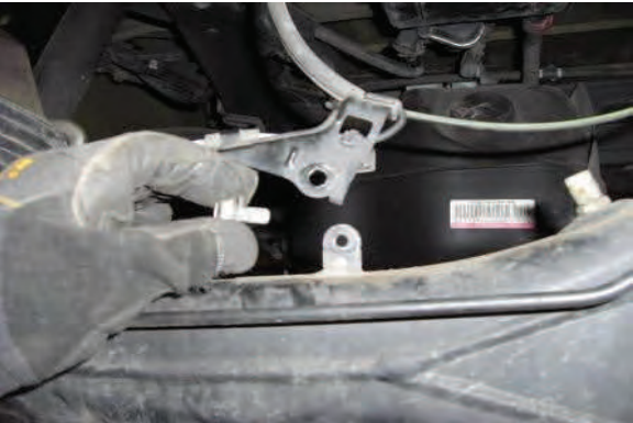
Disconnect ABS wiring brackets from axle.
