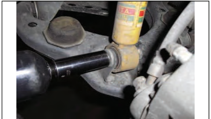
Disconnect lower strut mounting hardware
