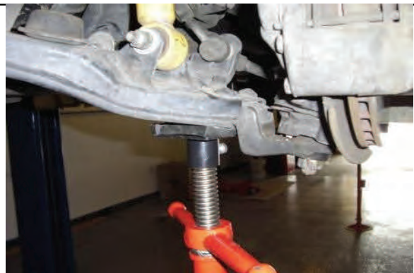
Raise lower control arm and attach lower strut mount
