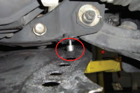
4WD Reattach skid plate with provided spacers and hardware
