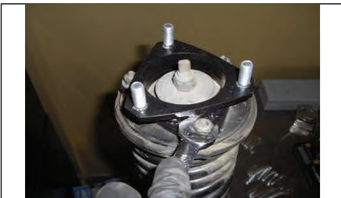
Attach new strut extension with OE hardware
