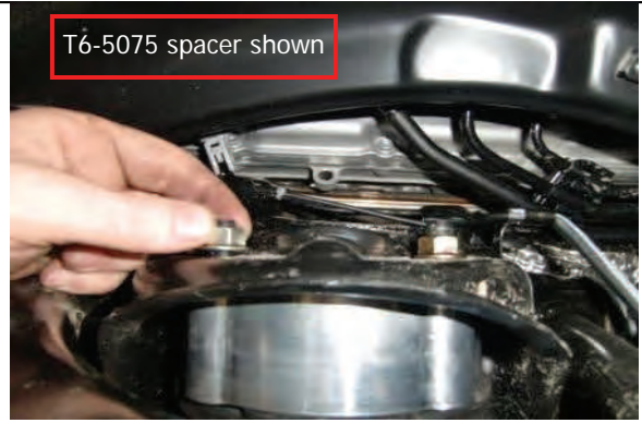
Reattach upper strut mount with provided nuts and tighten
