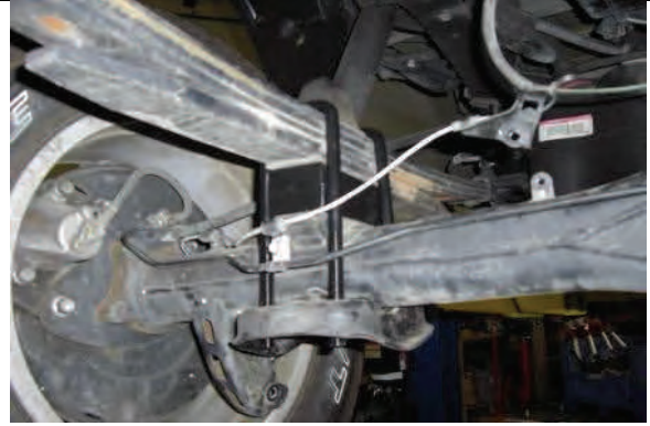
Attach lower mounting plate with provided hardware.
