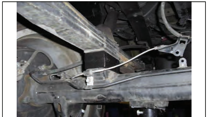
Raise axle and ensure locating pins are properly aligned.
