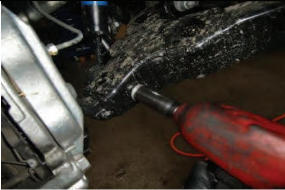
Reattach and tighten lower strut mounting hardware
