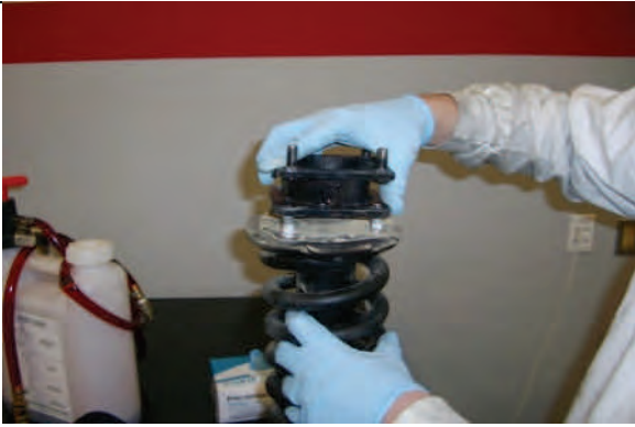
Attach strut extension spacer with OE mounting hardware
