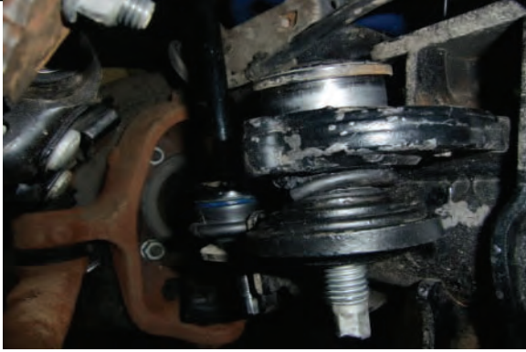
Remove ball joint from axle.
