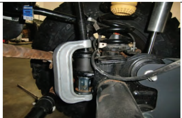
Use press tool to draw clevis into position
