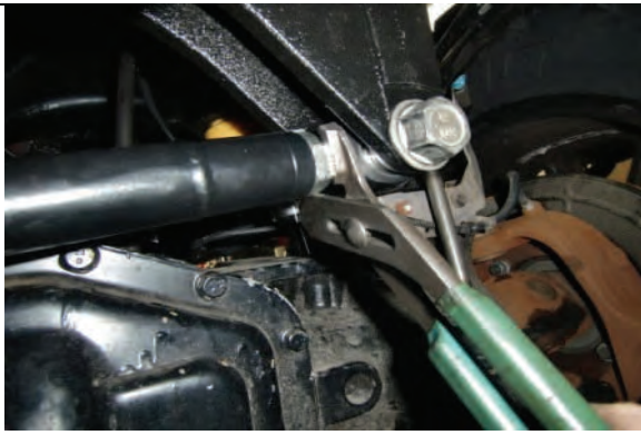
Tighten jam nut at frame mount
