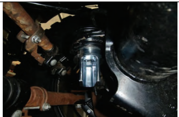
Align clevis so it lines up with track bar frame mount bracket
