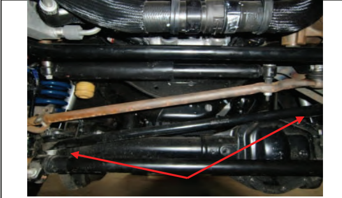
Front view of suspension, Track bar attaches to frame & axle
