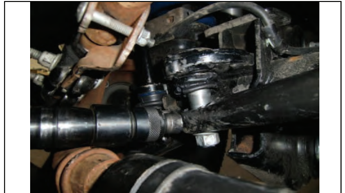
Use ball joint fork/air hammer to separate bar from ball joint
