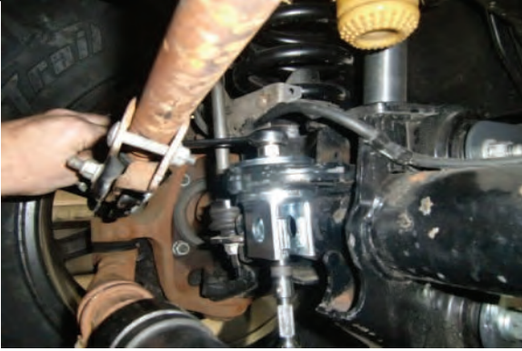
Tighten hardware to spec once clevis is properly seated
