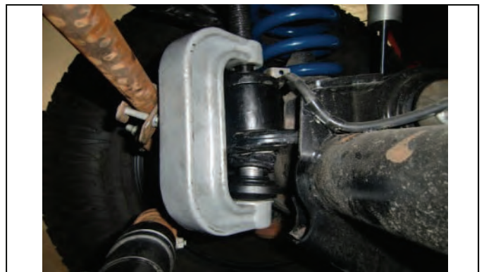
Shown, tool set positioned to remove ball joint
