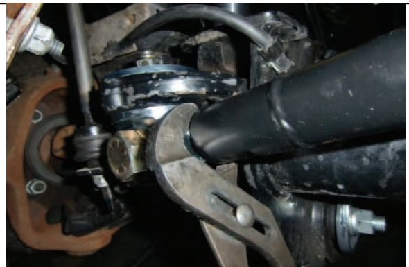
Tighten jam nut at axle mount
