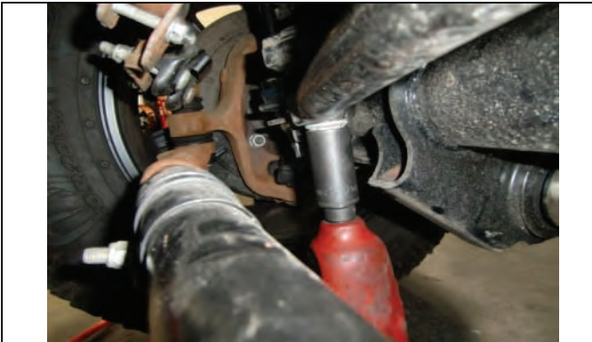
Loosen ball joint nut and leave attached
