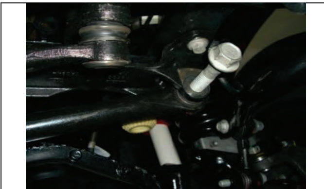
On opposite end disconnect hardware and remove bar
