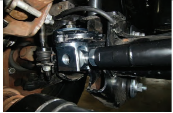
Insert track bar into clevis, check clearance.
