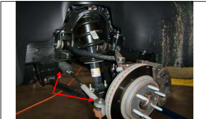
Photo shows inner/outer tie rod assembly
