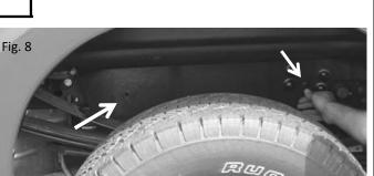
**7.** Re-install the screws and nuts that holds the rod to the bottom of the wheel fender (Front and Rear) (See Fig. 6)
