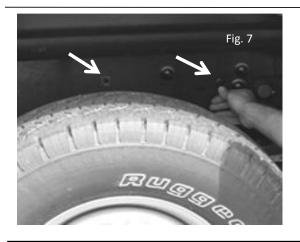
**9.** For the passenger's side: Repeat steps 2 - 7 using the Inner Wheel Well Liner marked (PS)
