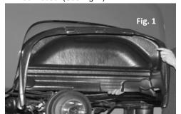
**3.** Be sure that the upper section of the plastic liner is mounted behind the flange and around the wheel well house edge. (See fig. 2)
