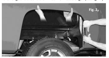
4. Be sure that the 3 holes drilled on the plastic liner are aligned with the 3 pre-drilled holes on the top edge of the wheel house, and install one plastic push pin in each hole. (See Fig. 3)
