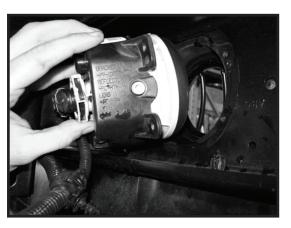
5. From the front of the vehicle, check to make sure O-rings are properly seated between the Euro Guards and the bumper.
