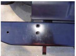
Note: Please keep all mounting bolts as they will be reused. A size 55 torx bit will be needed to remove original mounting bolts from vehicle.
