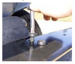
After the new bumper has been installed on the front of vehicle, hand tighten all bolts into place. Using the torx bit, tighten all bolts to secure bumper to frame. If installing new tow hooks used supplied hardware for upper mounting holes.
