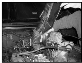
2. Remove rubber grommets from the air filter housing. Mount and install Heat Shield in place using 1/4-20 hardware.
