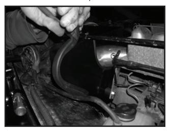
7. Attach the breather hose to the Intake Tube and to the valve cover using 1-1/16" tube clamps. Attach charcoal box breather hose to Intake Tube.
