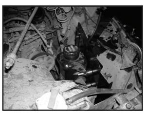
5. Install small end of Rubber Elbow onto throttle body using supplied #40 Hose Clamp. The Rear Intake Tube can than be installed onto the large end of the Rubber Elbow using a #48 Hose Clamp. On the end of the rear intake tube, install the Rubber Tube Coupler using a #48 Hose Clamp. Place the #56 Hose Clamp on the large end of the Rubber Tube Coupler to prepare for the installation of the Front Intake Tube.
