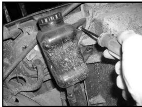
3. Remove hose connecting the power steering fluid reservoir to the steering box. Replace it with the longer Power Steering Hose supplied and secure with 1/16" Hose Clamps. Install Edge Trim onto Heat Shield and trim to length. Install Rubber Isolator Mount into slot in the Heat Shield using supplied M8 hardware.
