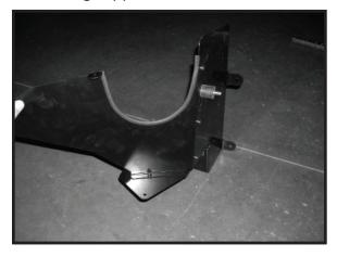
4. Install Heat Shield by inserting the two tabs behind the radiator shroud. Use the factory Phillips head screws removed in step 2 to reinstall the shroud and Heat Shield. Secure the bottom of the Heat Shield to original air filter housing bracket using the provided M6 hardware. Relocate the power steering fluid reservoir to the provided mounting location on the heat shield. Check all hoses for clearance around Heat Shield. Use provided 1/4-20 hardware and metal (2) Spacers for installation.
