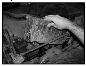
2. Remove rubber grommets from the air filter housing bracket. Remove (2) Phillips head screws from radiator fan shroud. If vehicle has power steering remove the flat head screw securing power steering fluid reservoir in place. For easier installation, unbolt front end of radiator support rod and rotate out of engine compartment.
