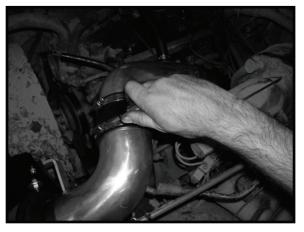
7. Attach the breather hose to the Rear Intake Tube and to the valve cover using 1-1/16" Hose Clamps. Attach charcoal box breather hose to Front Intake Tube. Also, reattach radiator support rod to its original location and use supplied Zip Tie to attach tab of Heat Shield to radiator support rod.
