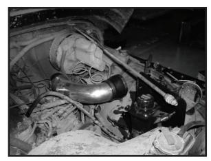
6. Prepare Front Intake Tube for installation by attaching the Air Filter to the end with the slotted bracket using # 56 Hose Clamp. Attach Front Intake Tube to the Rubber Tube Coupler with the #56 Hose Clamp installed in step 5. Use M8 Nut to secure bracket of Front Intake Tube to the Rubber Isolator Mount. Adjust Air Filter attachment for clearance if necessary. Note: This filter is polyester synthetic and never needs to be oiled. It can be cleaned with warm water and mild detergent dish soap.
