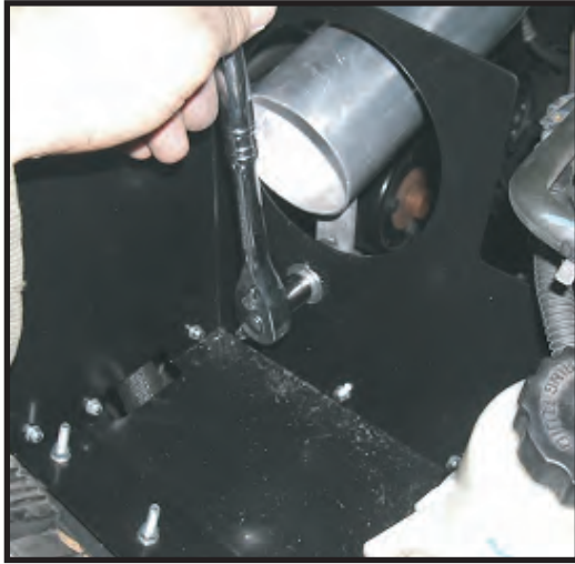
Secure tube to heat shield
