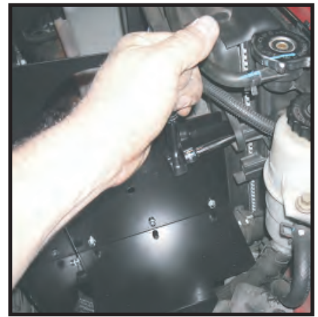
Tighten all heat shield bolts
