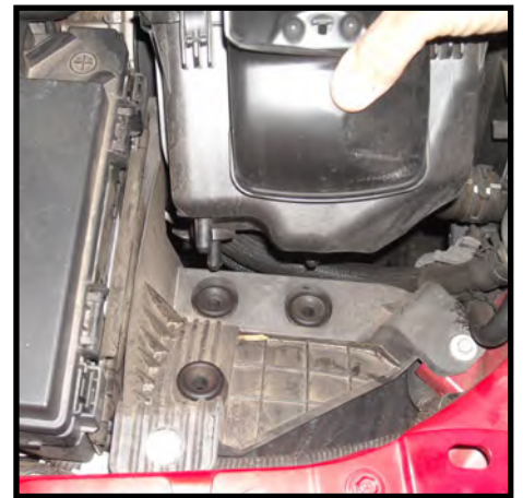
Pull air box free from inner fender
