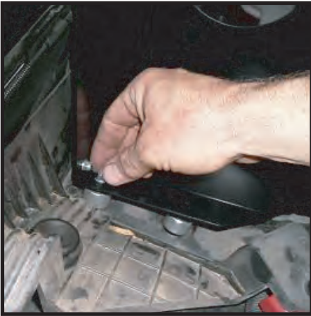
Place heat shield over spacers
