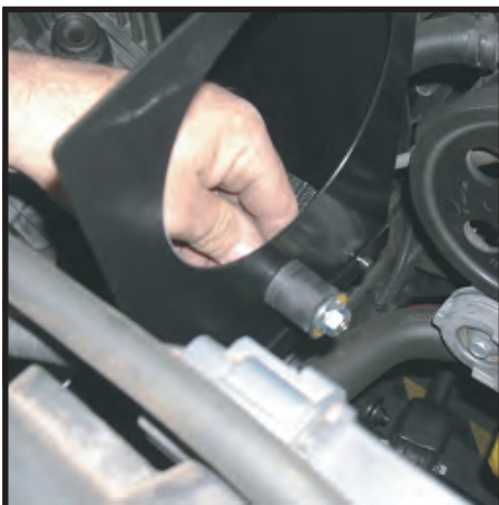
Isolator attached to heat shield
