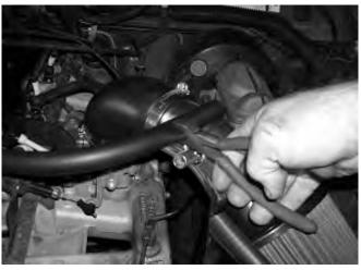
7. Secure the small vacuum line with a zip tie as shown. Attach the breather hose to the charcoal canister.
