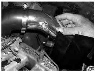
5. Secure intake tube to the rubber isolater mounted on the heat shield with nut and washer.
