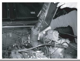
2. Mount the heat shield in place using the original mounting hardwaresaved in step 1.
