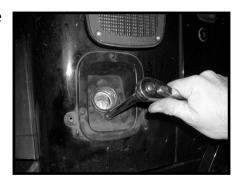
3. Remove the nut from the bracket holding the exhaust pipe in place on the passenger side of the vehicle. This will allow movement in the exhaust pipe during removal of the tank from the vehicle.
