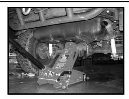
7. Remove the nuts holding the straps to the OE skid pan. Reinstall these straps in the RR skid plate using the square cutouts in the front of the pan. Remove gas tank from OE skid pan and place into the RR skid plate. Locate the proper slots in the rear of the RR skid plate for each straps threaded stud. Tighten the nuts onto the studs to secure the gas tank to the RR skid plate. Be careful not to over tighten these bolts.
