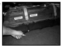
8. Position floor jack under vehicle with gas tank assembly centered on top. Slowly raise into position being sure to guide filler assembly to its appropriate location. The gas tank assembly may need to be tilted back to avoid the rear track bar when lifting. Stop about 3 inches away from the skid plates mounting position and reconnect the fuel rail to the top of the tank. It may be easier to reconnect the vent tube to the rollover valve and the electrical connector at this time also.
