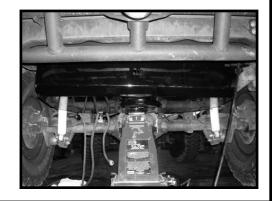
9. Resume lifting the gas tank assembly slowly into position. Line up factory mounting studs with the slots in the skid plate. Tighten the 7 nuts onto the factory studs evenly to 17 ft-lbs to secure gas tank assembly into position. Reconnect the high pressure fuel line, evaporation hose, and electrical connector (if not already connected in step 8).
