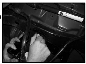
5. Install Front Bracket by replacing bolts removed in step 2. Do not tighten as assembly will have to be adjusted when skid plate is installed.
