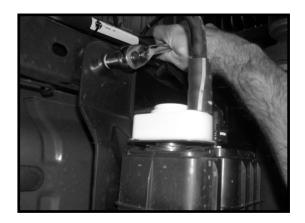
3. Slide Rear Bracket over the rear of the vapor canister toward the front of the vehicle being sure to keep the canister from hanging. It might be easier to have a partner hold the canister while sliding on the bracket.
