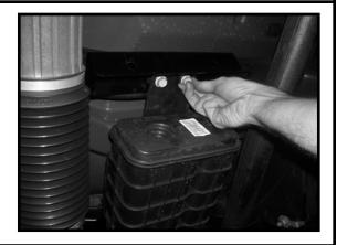
5. Fasten Skid Plate to brackets installed in steps 4 and 5. Adjust brackets and vapor canister if necessary to line up holes. Push Skid Plate up as far as it will go when tightening.
