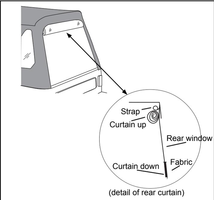
**Rear Window:** To roll up the Rear Curtain, start at the bottom and roll it upward toward the inside of the vehicle. Avoid wrinkles in the fabric and window. Secure the window in place with the curtain straps inside of the top.
