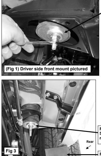
To prevent the factory center bolt from spinning, hold the center bolt with a wrench as you loosen or tighten the factory hex nut. Do not remove the center bolt or the rubber body mount.
