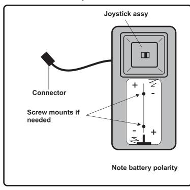
\*Be sure to check the polarity of the batteries if the control fails to operate the mirror after the installation.
