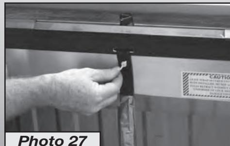
**C.** To open the Cover, pull back slightly on the Handle to relieve spring tension from the Latch Mechanisms and turn the Lock Lever to the 10 o'clock (unlatched) position.
