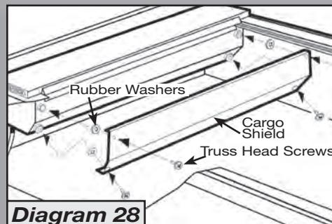
**D.** Use 1/4 - 20 x 1/2" truss head screws and rubber washers to secure the Cargo Shield (*Diagram 28*). **Note: The rubber washers go on the inside of the Cargo Shield.**
