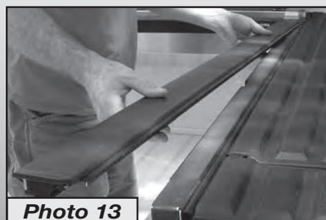
Flanges (*Photo 13*) and key them into the Housing Stems (*Diagram 14*), being sure that the Handle is properly engaged into the Tracks.
