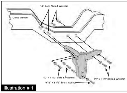
7. Install the supplied 1/2" x 1 1/2" bolts, washers, & nuts labeled as "**B**", through the new Skyjacker bracket & cross member. Pivot the bracket down so the tab is flush against the cross member lip. Drill a 7/16" hole, for bolt labeled as "**C**" & install the supplied 7/16"x 1 1/2" bolt, washers, & nut
