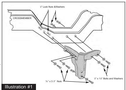
**"Existing-A"** on illustration). Note: the original two holes labeled as **"Existing-A\*"** are for the existing two bolts on the back of drop bracket. Be sure to install original hardware in these two holes, and tighten.
