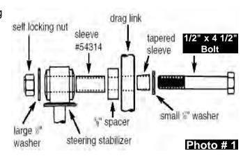
8. Attach the body end of the new Skyjacker steering stabilizer into the OEM mount using the OEM hardware & tighten.
