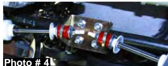
7. Attach both of the new Skyjacker steering stabilizers to the new outer brackets & main bracket. (See Photo # 4 & # 5)
