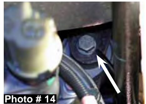
REAR mounting point on passenger side diff tube.
