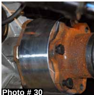
Driver side shown with 3.35" cv-shaft spacer.
