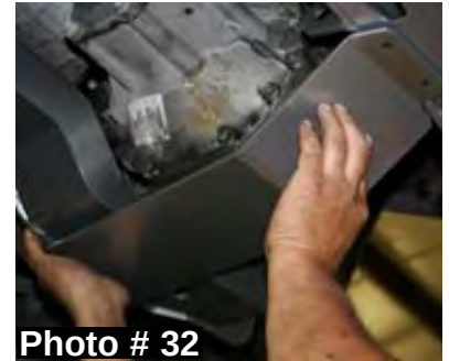
Passenger side shown with one 15/16" C.V. spacer.
