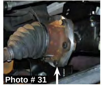
Passenger side shown with one 15/16" C.V. spacer.
