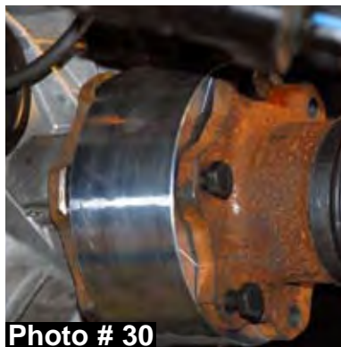
Driver side shown with 3.35" cv-shaft spacer.
