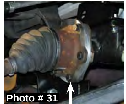
Passenger side shown with one 15/16" C.V. spacer.
