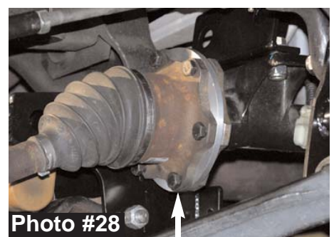
Photo #28 Passenger side shown with one 15/16" C.V. spacers.
