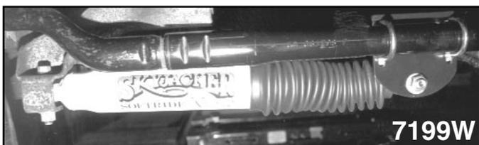
Insert 1" long spacer, at new drilled hole, inside the original mounts. Insert 9/16" x 3" bolt with washer thru spacer and tighten locknut. Reattach track bar using original hardware (Photo #2). Completely tighten all hardware.
