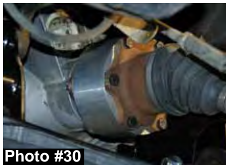
Driver side shown with 3.312" C.V. spacer.
