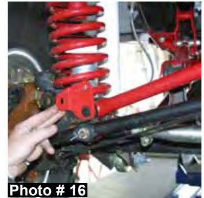
5/16" x 3/4" thread cutter flange bolt.
